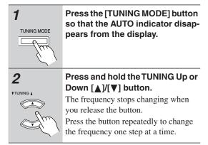
Frequency changes in 0.05MHz steps for FM and 9kHz (or 10kHz) steps for AM.
